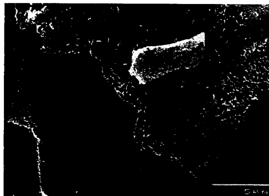
Fig. 3. Carbon deposition on beryllium.
